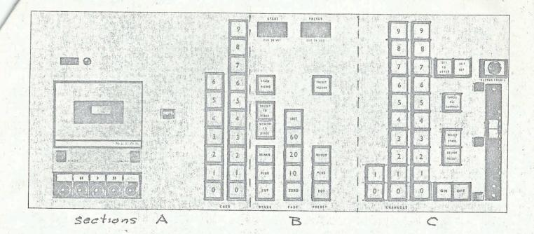
For ease of operation, the controls have been arranged in two basic groupings representing those required for rehearsal and those for an actual show. All push-buttons illuminate when depressed, the preset functions showing as blue for ease of identification.
